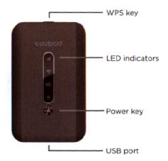
**Power key:** Hold the Power key for 3 seconds to power device on/off.
